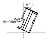
B. Clean the filter with a vacuum cleaner or wash it with clean water and dry with a dry cloth.
