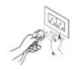
1.2 Make sure the plug is placed fully & firm into the socket!
